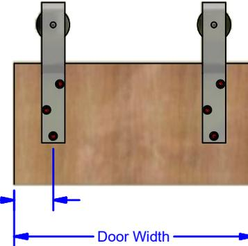
Edge of Door to Center of Hanger (5 7/8 Min. for Bi-Parting Applications)
