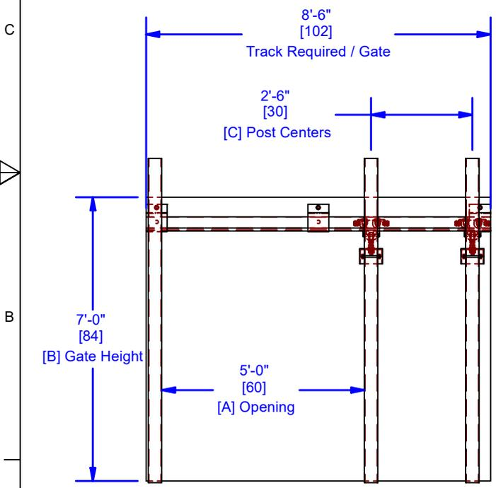
**Gate Closed-Interior Elevation**
