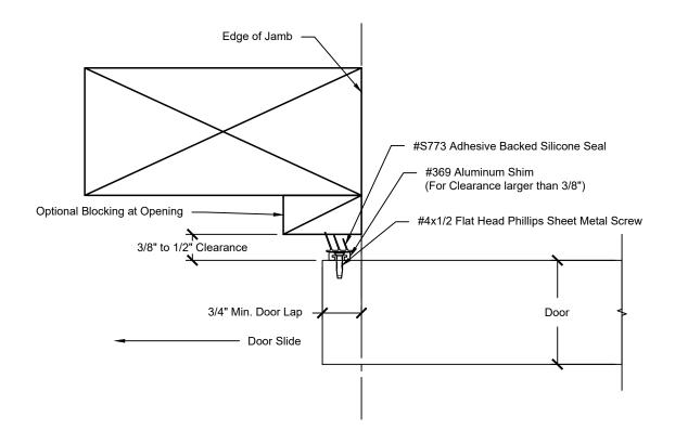
Jamb Plan Section Detail: S773 Silicone Adhesive Seal
