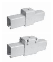
The **5PX18** bracket is used only for suspending #5 track by means of a single bolt. The bracket should be used for supporting the track when the joints are welded and should be used on curves except when the track is supported by angles or flat bar. Distance from top of bracket to bottom of track is 3-3/4". Finish: Painted. Weight: 2 lbs.
