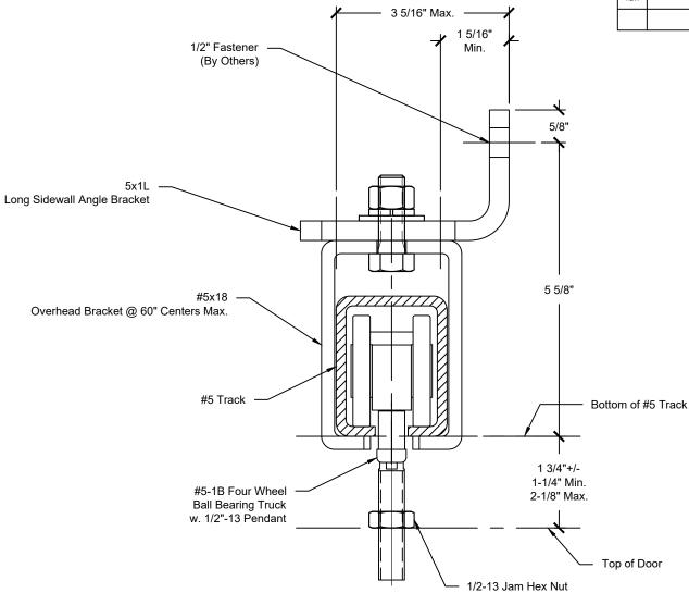
5-1B Sidewall Detail w. 5x1L Long Bracket
