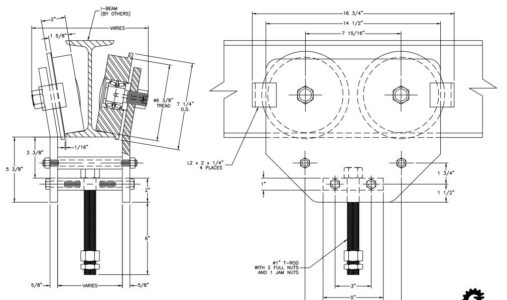
DWG #0001967 STOCK PART #CR-2T DESCRIP: 2 TON I-BEAM TROLLEY (4,000 LBS CAP) {SPECIFY BEAM} DRAWN:BCM 11-3-01 REV:----SCALE: None SHEET # 1
