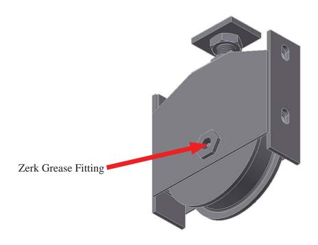
Access should be provided to the zerk grease fitting located on the face of the bottom roller as depicted above. Every (1) Year grease should be reapplied depending upon use.
