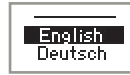
Select your language before entering the first LCD menu. During the first 30 seconds after power-on of the sensor or later in the diagnostics menu.
