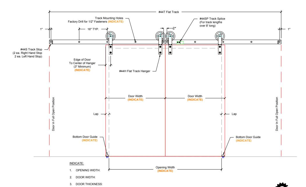
44 FLAT TRACK **DWG #44H DESCRIP: 44H ELEVATION- BIPARTING** DRAWN:BCM 8-14-08 SCALE: NONE SHEET # 1
